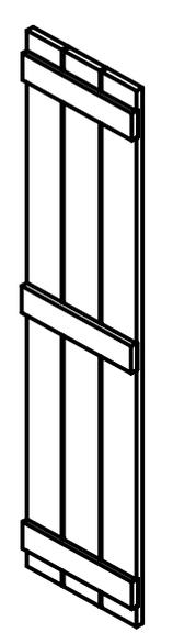
3 Vertical Boards and 3 Horizontal Battens
