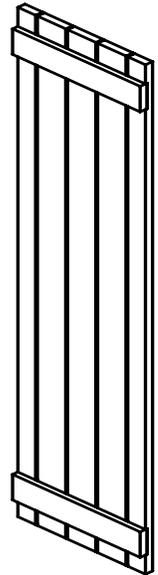
5 Vertical Boards with 2 Horizontal Battens
