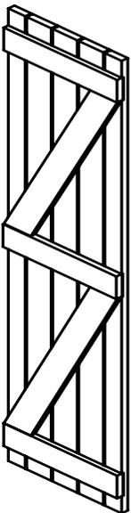
5 Vertical Boards and 3 Horizontal Battens Double Z-Board
