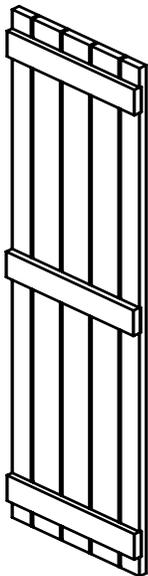
5 Vertical Boards and 3 Horizontal Battens
