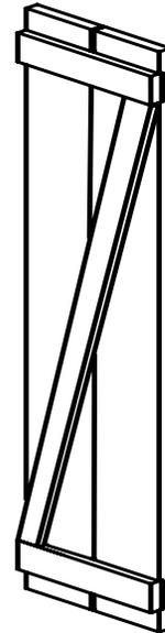
2 Vertical Boards with 2 Horizontal Battens with Single Z-Board
